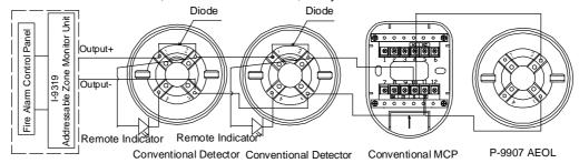
2. When the detector is connected with a conventional fire alarm control panel (those within the dotted line are equivalent to a conventional fire alarm control panel) or an I-9319 Addressable zone monitor unit in series, if an end of line resistor is connected to the end of output loop, then no diode is connected to the detector base. The system connection is shown below:
