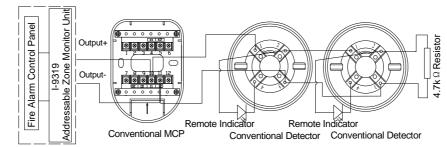
Maximum 15 detectors can be connected in one zone. Cooperating with end of line device, the compatible panel can monitor the cable for open circuit and short circuit. Panel will report if any detector is removed. With the AEOL, the functioning of other device will not be affected by the detector removal.
