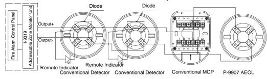
When the AEOL is not used as the detector base, a cover should be added, the system connection is shown below:
