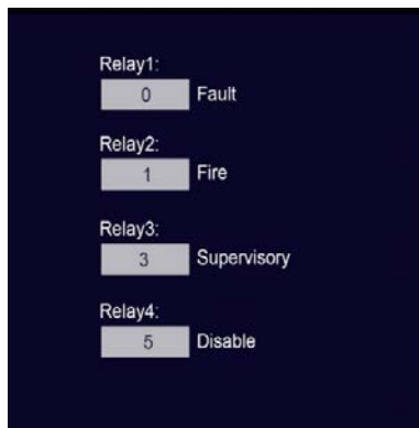
Figure 77: 1 Relay Output Setup
